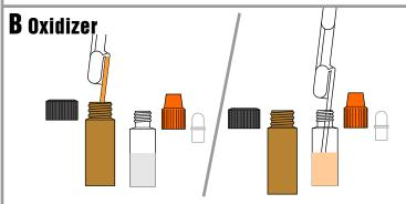
Using a 100 ul volume pipet, remove 200 ul (2 X 100 uL) of oxidizer from the amber serum vial and add to the orange cap dropper bottle by removing the orange cap and dropper tip. After adding the 200 ul into the bottle, put back the dropper tip and orange cap on the bottle and mix by shaking moderately.
