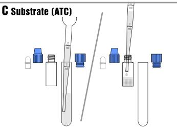
(3) Substrate (ATC) Using a 3ml transfer pipet remove, 2 ml from the blue cap test tube, add to the blue cap dropper bottle by removing the blue cap and dropper tip. After adding the 2 ml into the bottle put back the dropper tip and blue cap on the bottle and mix by shaking moderately.
